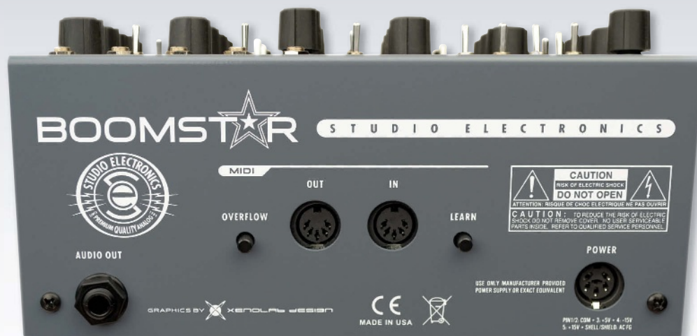
Left to right: Monaural audio out, Overflow button for chaining multiple Boomstars polyphonically, MIDI I/O, Learn button for changing MIDI receive channel, and power supply jack.
